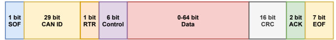
Fig. 1: Frame format of an extended frame CAN message that uses a 29-bit CAN ID.
