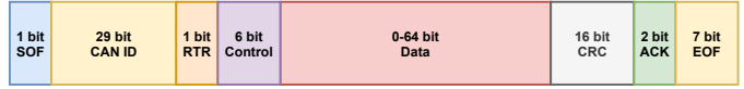
Fig. 2: Frame format of an extended frame CAN message. In the case of a standard CAN message, the ID field contains the 11-bit identifier.
